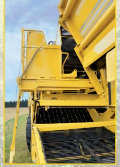
Working platform, 300 mm extendable - immense working area allows freedom of movement
