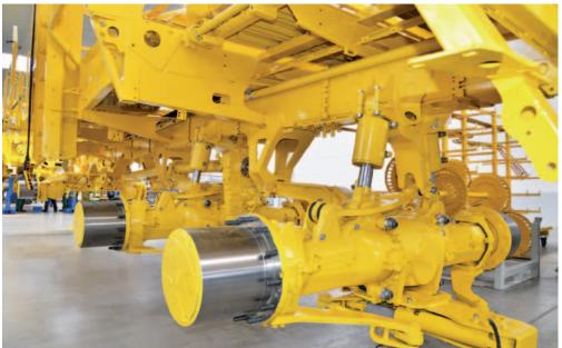
Hydraulic chassis, automatic slope compensation
