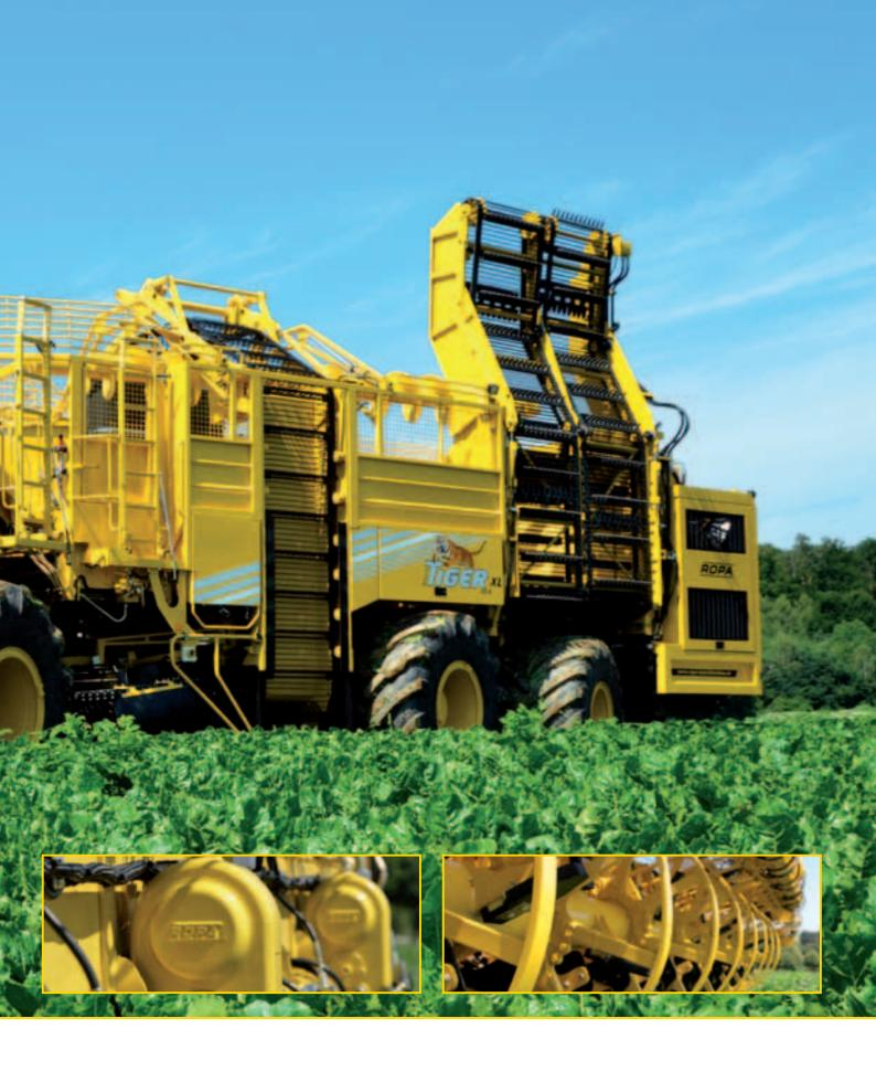
**load control** (with integrated suspension) guarantees optimum traction and load distribuion with, at the same time, an **outstanding manoeuvrability** in all harvesting conditions. The extra-wide 1050/50 R32 Michelin tires at the front axle ensure superior soil protection, even with a completely filled beet tank.
