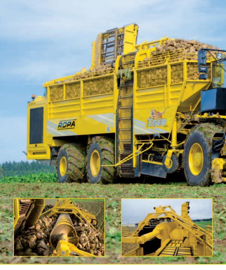
Beet tank of 40 m<sup>3</sup> capacity – flexible operation and sustainable soil protection
