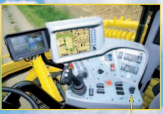
Multifunctional Terminal The complete Maus can automatically be folded in and out with only one control switch
