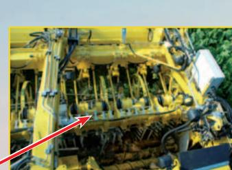
**Excellent view across the pickup unit** -> the operator overlooks the beet row and the operation of the micro-topper
