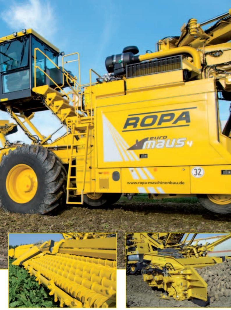
Separate drives for 3 groups of rollers with individual setting of revolutions and automatic reversing for stone protection
