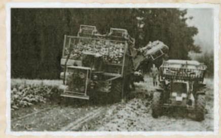
The new six-row comprehensive sugar beet harvester of the Paintner system (rear view) in operation.
