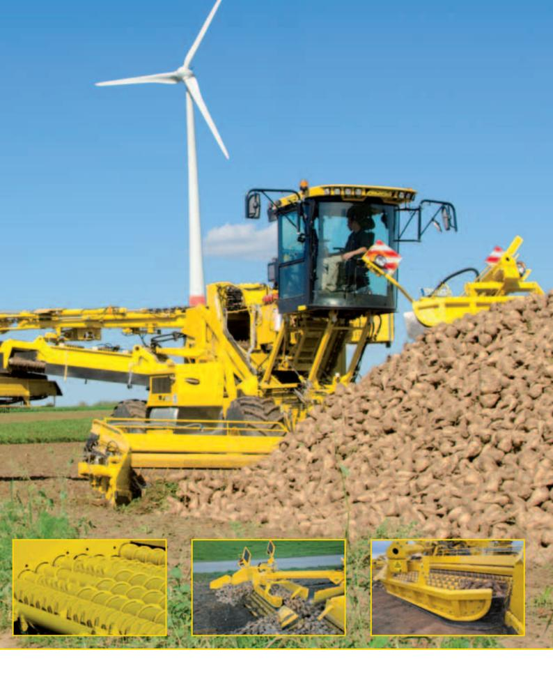
with protective helpers, brought onto the next spiral roller cleaners and travel into the center of the pick up. At the point of transition from spiral roller cleaners to the in-feed web hardened end plates cover, to protect the beet and to reduce the wear and tear, at the roller ends. The beet collector telescope arm (now 180mm x 180 mm x 5 mm) uses proportional control valves and is equipped with a plate with reinforced rubber lip and angled corners.
