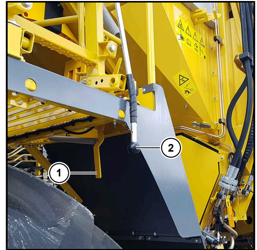
Ladder to driver's cabin in transport respectively working position
