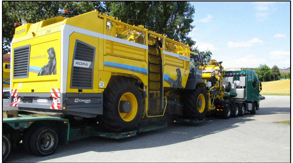
Regular low loader for road transport with minimum transport height
