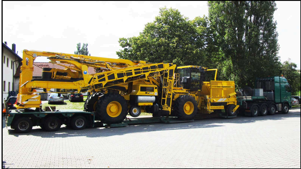
Regular low loader for road transport with minimum transport height
