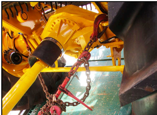
Lashing of the front axle
