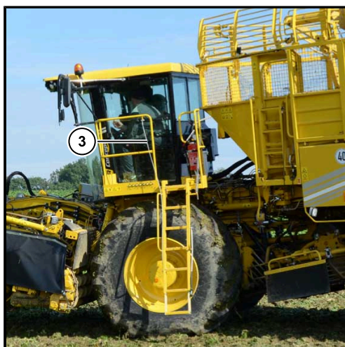
Ladder to driver's cabin in transport respectively working position
