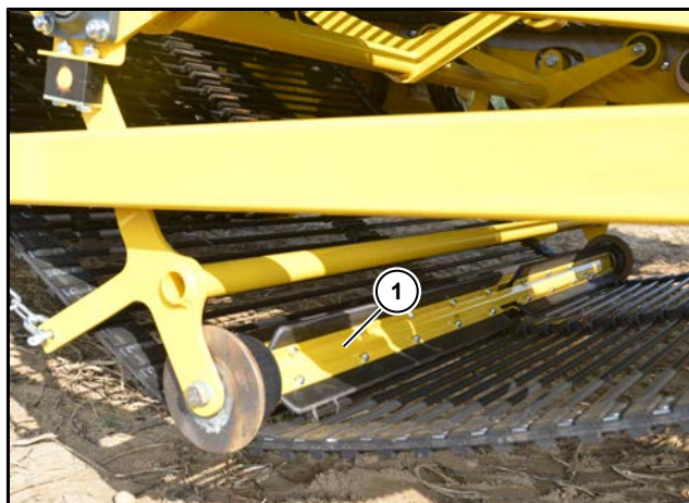
(1) Sieve conveyor 1 cleaning roller 2016 - 2020 model years
