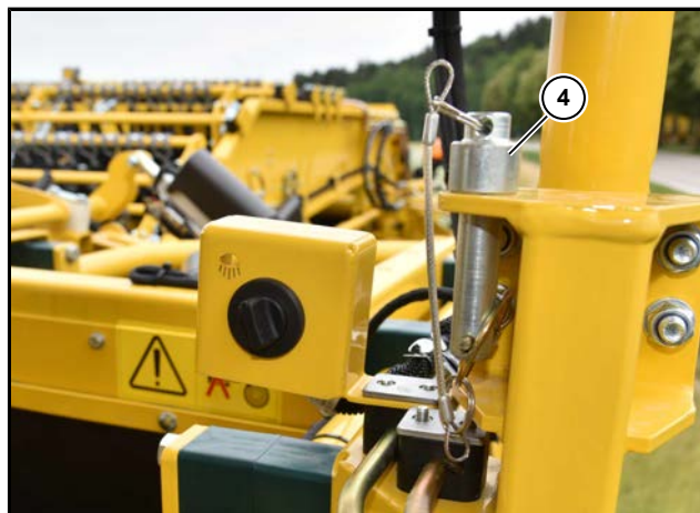
(4) Canopy safety bolt rear left in parking position
