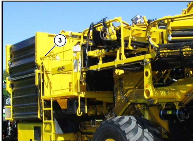
(3) Safety rail at the ladder left (till 2017 model year)
