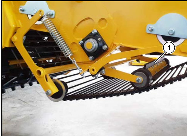
(1) Sieve conveyor 1 cleaning roller from YOM 2021
