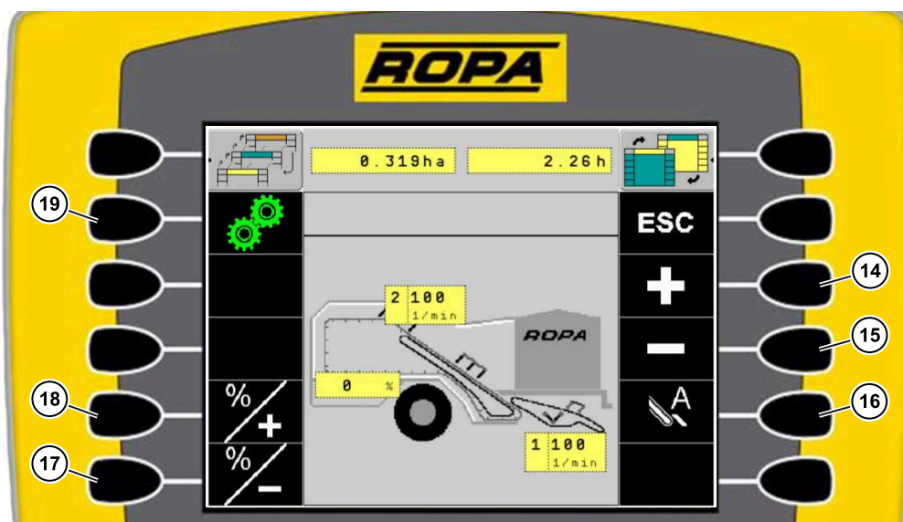
Sieve conveyors automatic function deactivated with synchronous adjustment
