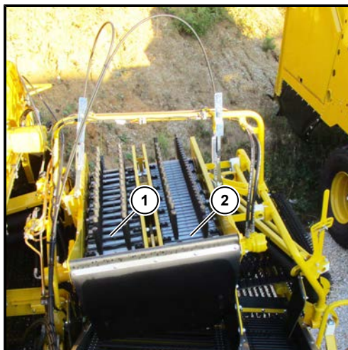
Mechanical height adjustment of UFK
