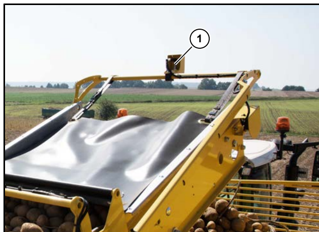
(1) Automatic filling ultrasound sensor
