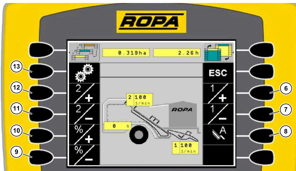
Sieve conveyors automatic function deactivated with individual adjustment
