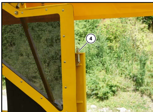
(4) Sunroof safety bolt left in parking position
