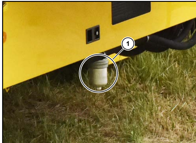
(1) Drive wheel suction filter
