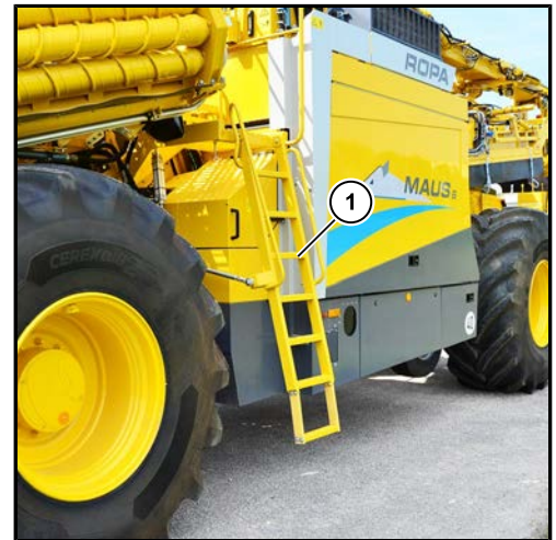
Ladder to driver's cabin in transport respectively loading position
