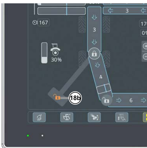
Counterweight arm lock at the end-stop
