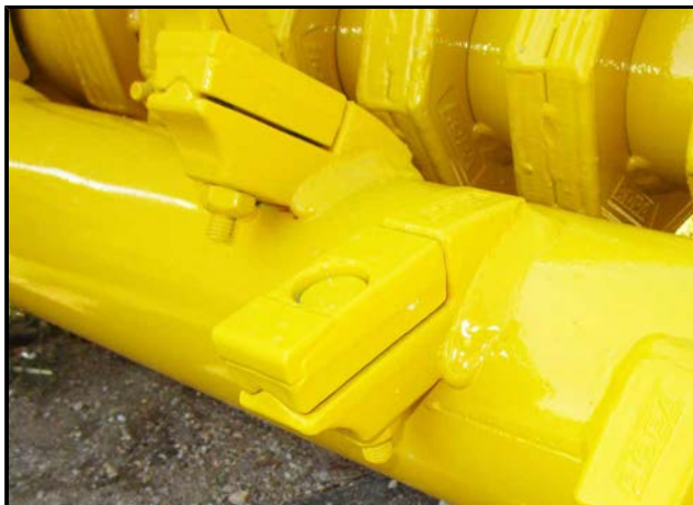
Pickup finger with wear plate
