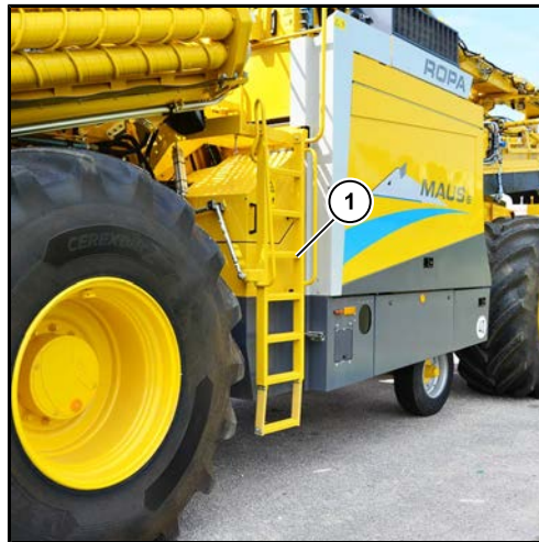
Ladder to driver's cabin in transport respectively loading position
