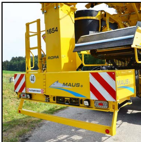
Auxiliary steps on the fuel tank in road position respectively folded for refueling
