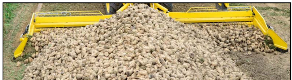
Incorrect setting of the clearing shields. Soil is shoved in the clearing shield area. Moreover, incorrect approach to the pile. It should be approached as centrally as possible. (Image of the previous model Maus 5)
