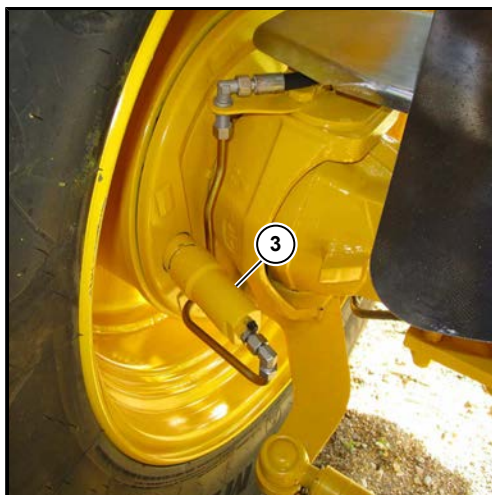
(3) Rear axle with hydraulically-actuated drum brake
