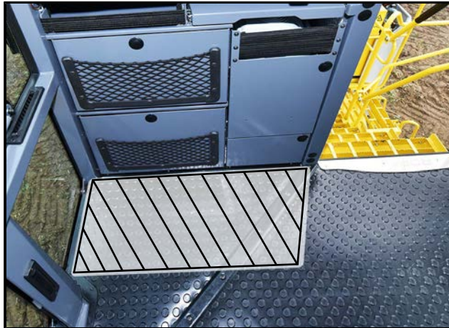
Non-heated area of the underfloor heating
