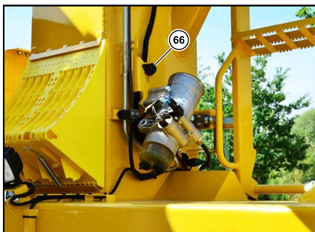
(66) Outlet on fuel tank 24V / 8A maximum
