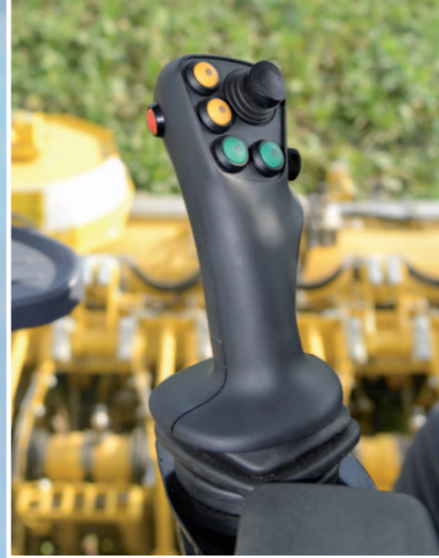
Control element on the left armrest for fine control of bunker unloading
