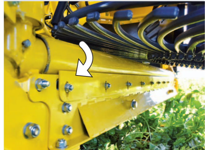
Rotating transition tubes at the elevator infeed prevent accumulation of soil
