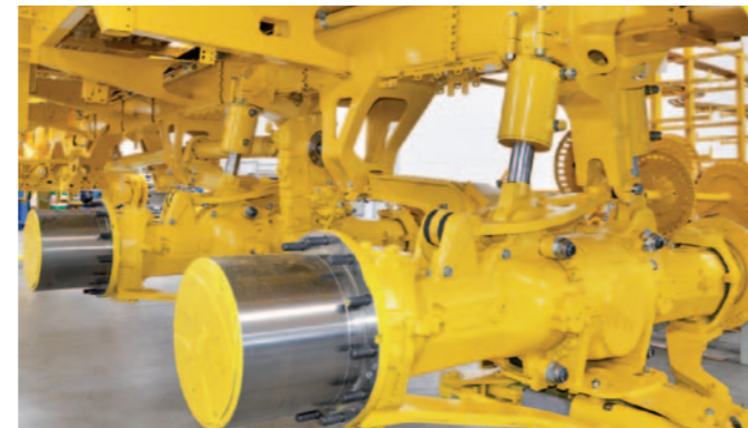
Hydraulic chassis, automatic slope compensation
