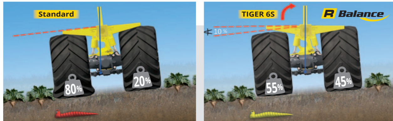
On the slope, the load and the gravity centre of the slope bottom side are shifted to the slope top side: soil-protective sugar beet harvesting also on the side slope!
