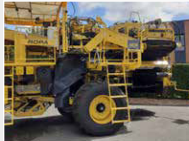
The Keiler 2 (German for “boar”) now boasts a new trash separation system; for the first time it has two finger combs that are arranged behind each other.
