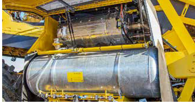
The emission cleaning system comprises SCR and particle filter (top) and a 400l tank for the spraying system (bottom).
