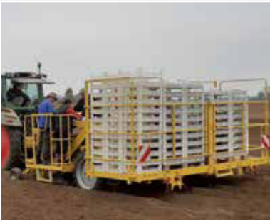
Ropa is currently testing a planter for chitted plant potatoes. Further machines of this type are to follow.
