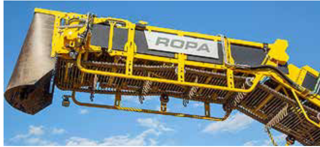
For improved weighing accuracy, two load cells measure the load on a separate frame.
