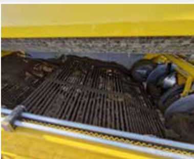
The pick-up on the Keiler 2 is now available with a split lifting web, a boon in heavy soil.
