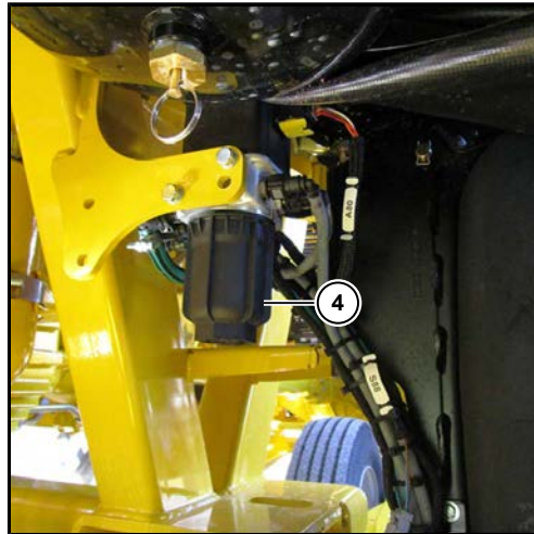
(4) Filterhus AdBlue® pumpemodul
