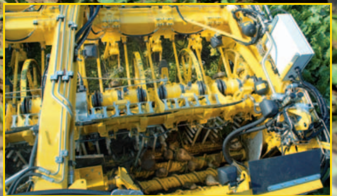
Excellent view across the lifting unit -> the operator watches the beet row and the operation of the Micro-topper
