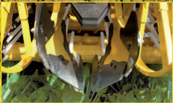
ROPA lifting share angle and distance are optimally adjustable to six positions for more careful beet treatment.
