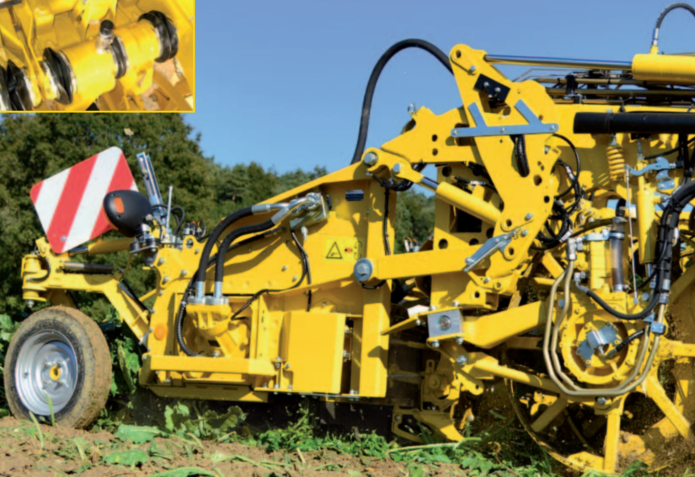
Hydraulic stone protection, positioned on top, maintenance-free linear guide
