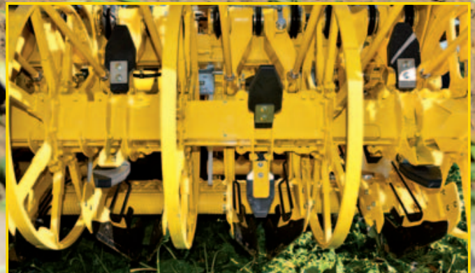
Depth control wheels with variable row width of 45/50 cm, adjustable with a button push from the cabin
