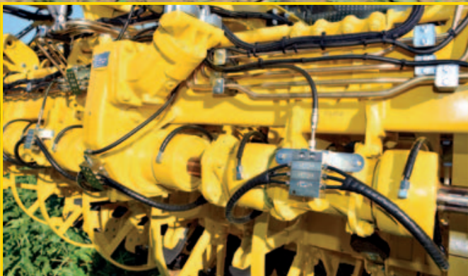
Faster oscillating share drive with axial-piston motor and spur gear, adjustable taper roller bearings.
